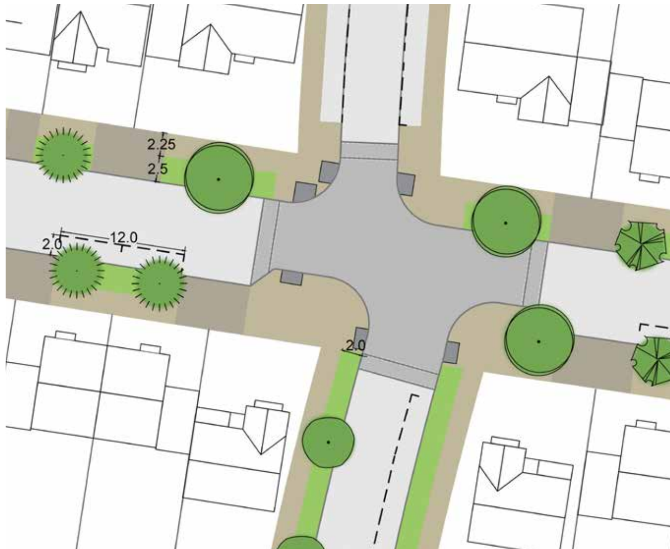
Figure 20: Diagram showing a typical neighbourhood junction with trees and their relationship with properties, parking spaces as well as tree-pit and verge sizes (dimensions shown in meters). These dimensions are considered best practice but not all locations will have ideal conditions, thus a discussion with the Local Authority and highways team should be carried out to find the best balance to ensure the street function and the longevity of trees.
