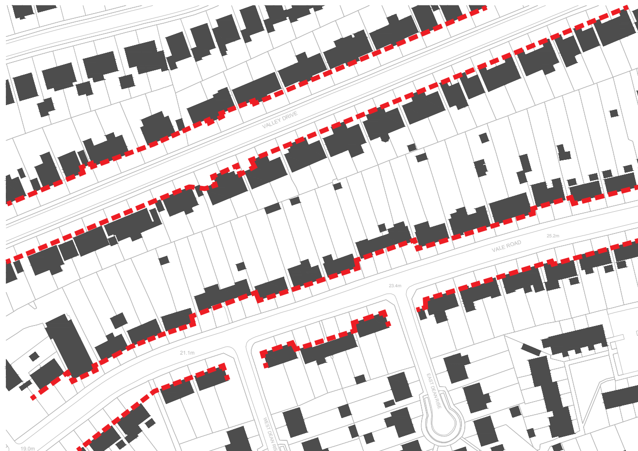
Figure 25: Example Map showing the typical consistent building line along Valley Drive & Vale Road. The dashed red line on the plan shows that small variations add interest to the streetscape but do not undermine the general building line along the street, thus preserving the townscape integrity.
