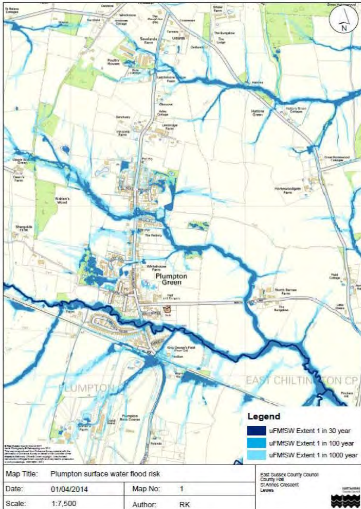
Map E: Updated Flood Map for Surface Water (uFMfSW). Included courtesy of East Sussex County Council, from data produced by the Environment Agency.
