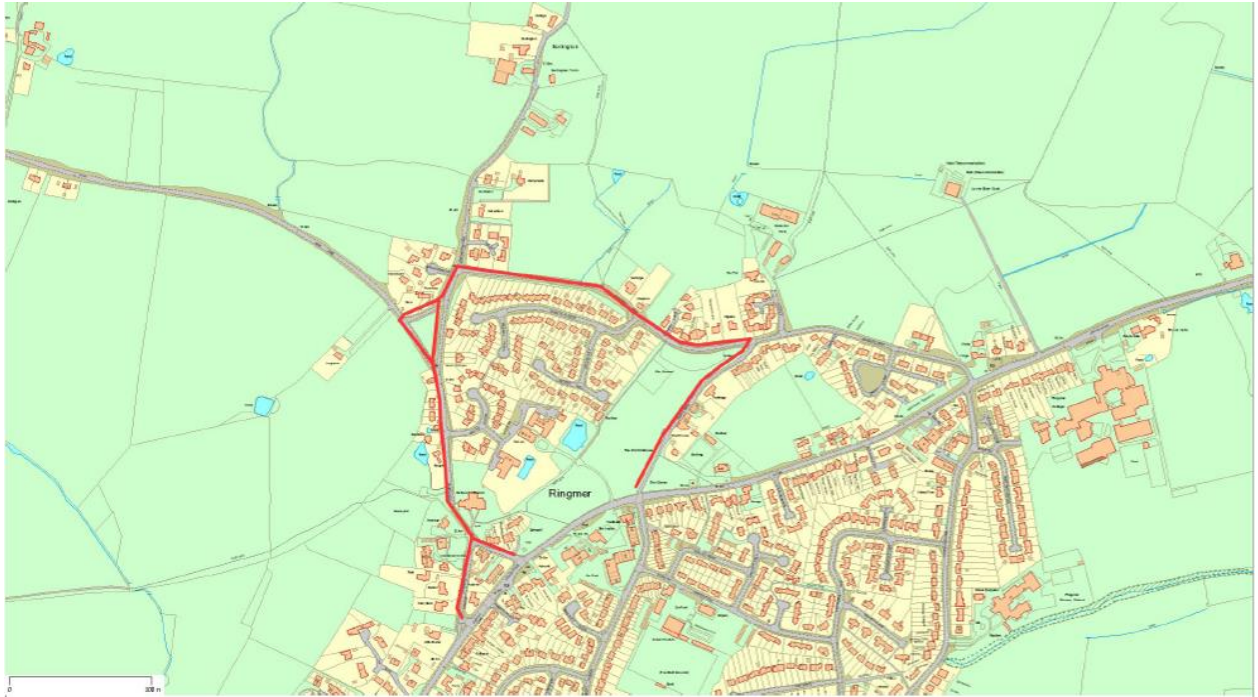
Map 8.1 Identified pinch points in the local road network are indicated in red
