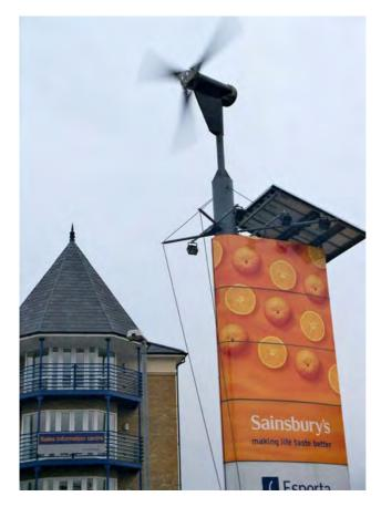
Turbines can be connected to the electricity grid via a meter so that the energy generated is offset directly against the building's electricity consumption. Assistance will be needed from the building's conventional electricity supplier in order to meet relevant electrical connection requirements.
