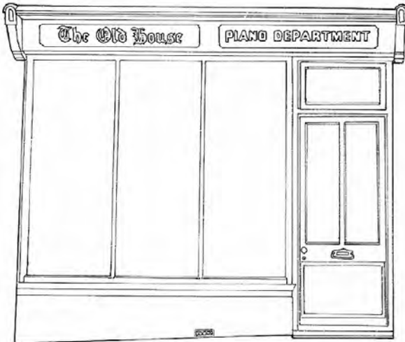
21 Church Street undecorated simple shopfront with a well proportioned fascia
